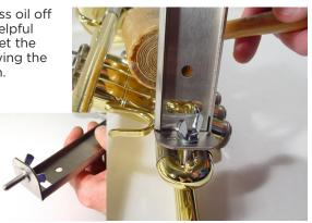
with the wing nut to the small end of the handle as shown in the picture, place the pin in the crook and tap on the handle with a broad faced light weight mallet. A plastic or rawhide mallet works well here.
