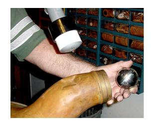
The Skyhook rotates 360 degrees, allowing you to work with both hands free to direct your work using your upper body and weight strength to remove dents.
