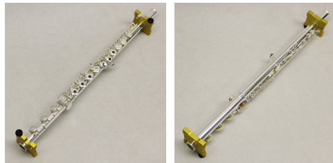
Fig. 4-5: Rotating the Flute Blocks allows 360° access.
